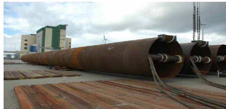
Length: 50 m, Diameter: 2,70 m, Weight: 160 t
